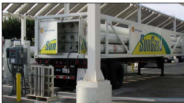
Figure 19. Hydrogen Tube Trailer
