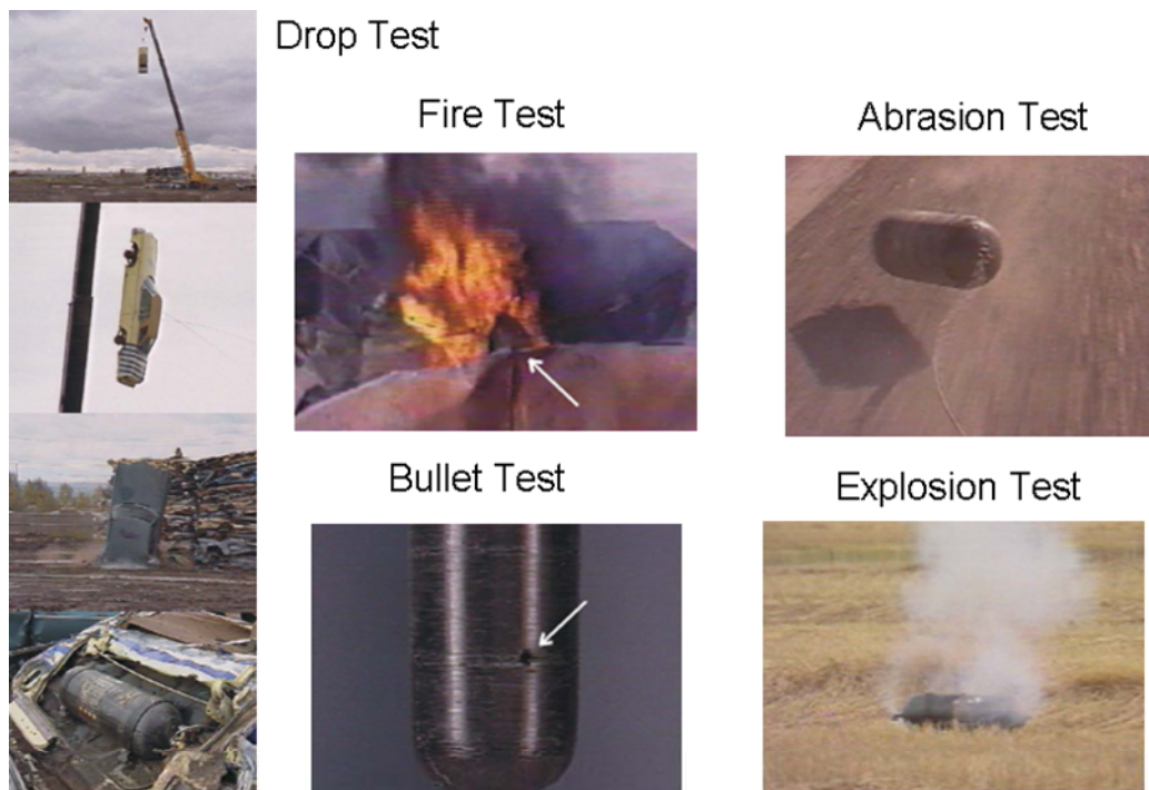
Figure 14. High-Pressure Storage Vessel Qualification Tests
